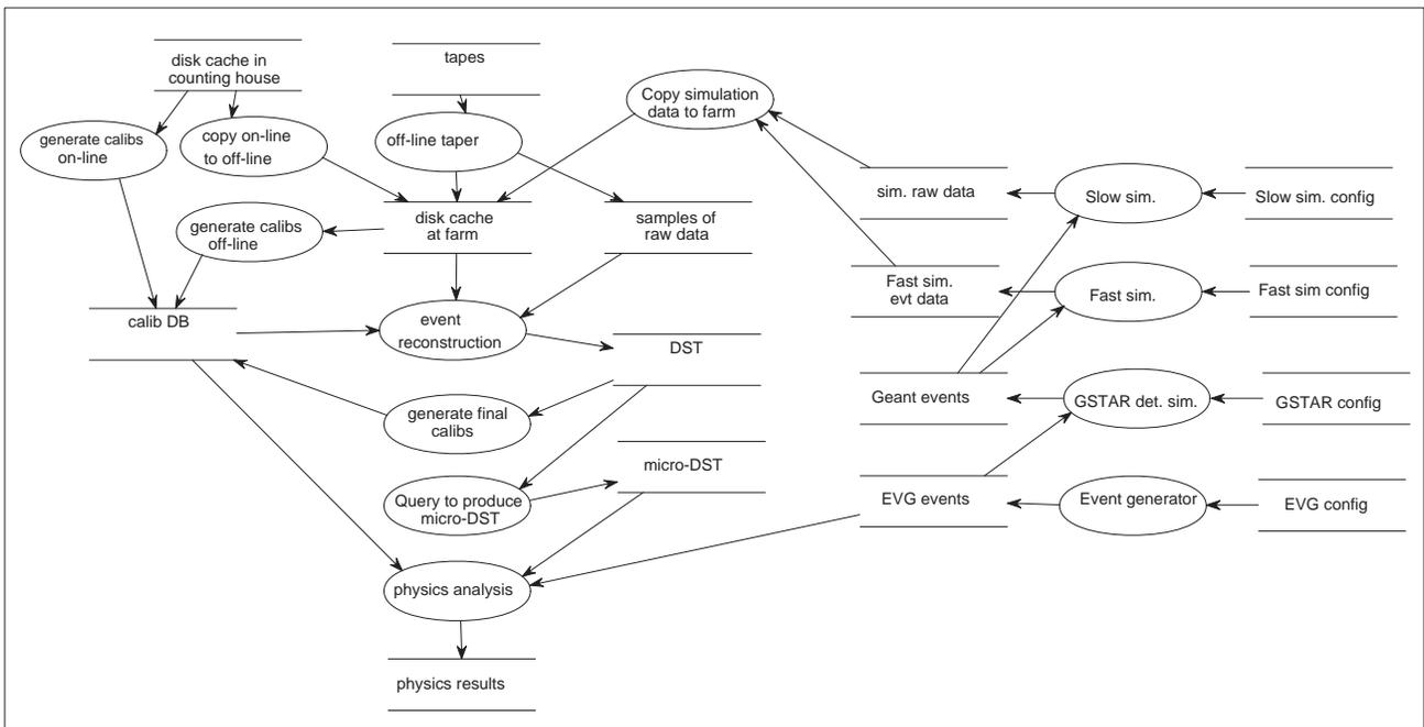
Figure 4: Data flow diagram of STAR Off-line Processing. See itemized descriptions in Tables
