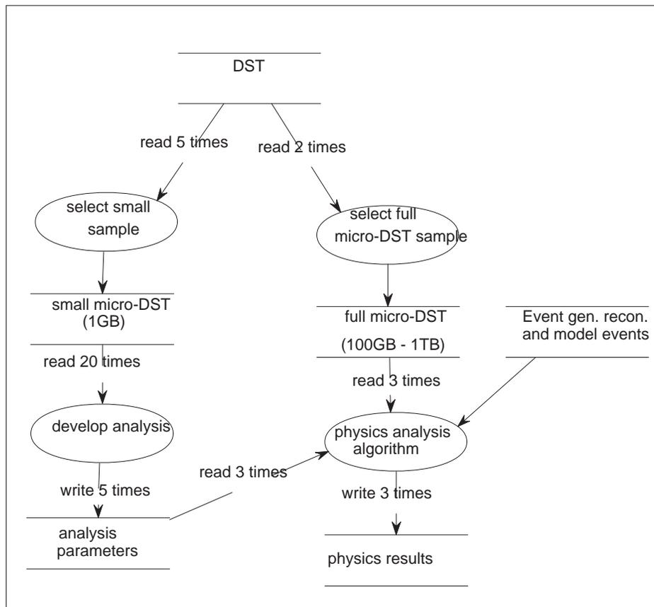
Figure 5: Detailed data flow diagram of STAR Physics Analysis. This activity is commonly called data mining.
