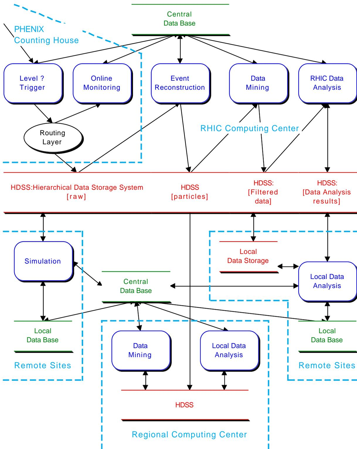
Figure 3: A pictorial view of the PHENIX Computing Model. Please refer to the text for details.
