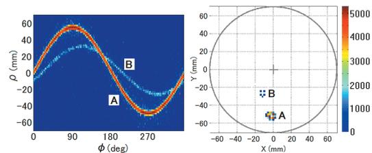
Fig. 3. Sinogram (left) and reproduced image (right) where the circles show the turntable and the RI sources.
