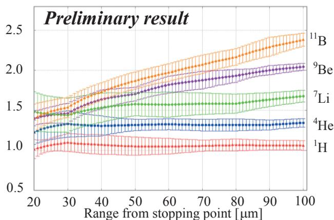
Fig. 2. Volume ratio for each nuclides ( $\theta = 75^\circ$ ) to  ${}^1\text{H}$  ( $\theta = 90^\circ$ ).
