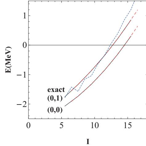
Fig. 1. Comparison of the excitation energy in the leading order approximation<sup>5)</sup> with the exact results as functions of  $I$ . The solid lines correspond to  $I - j = \text{even}$ , the red dashed lines to  $I - j = \text{odd}$ , and the dotted blue lines to the exact results. The attached numerals (0,1) and (0,0) correspond to quantum numbers of  $(n_\alpha, n_\beta)$ .
