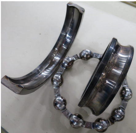
Fig. 1. Damaged bearing unit, disassembled from the coupling side of the motor unit.
