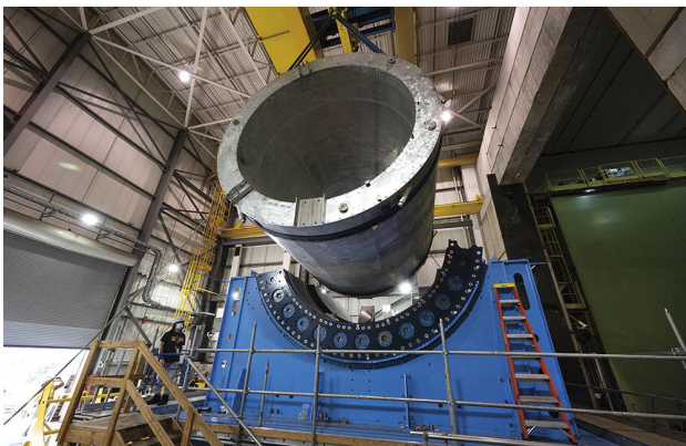
Fig. 1. The Babar magnet assembly on the bottom portion of the outermost detector, i.e. hadron calorimeters.
