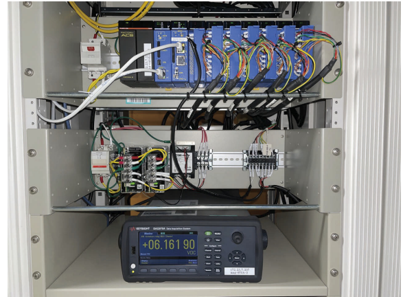
Fig. 1. Picture of a unit of the beam interlock system driven by changes in the magnet current (Curs-BIS).
