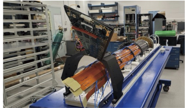
Fig. 2. The mock-up of a quarter portion of the INTT inner layer barrel assembled in BNL.
