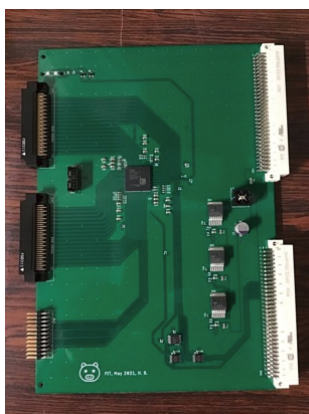
Fig. 1. Photo of the FPGA integrated TDC board.
