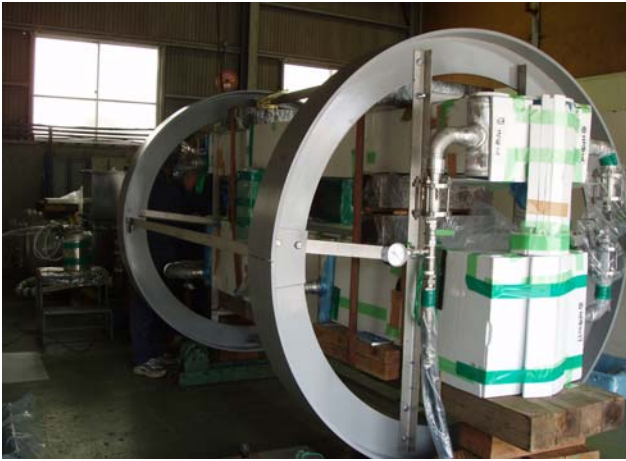
Fig. 2. Cleaning process of the heat exchangers in the factory.
