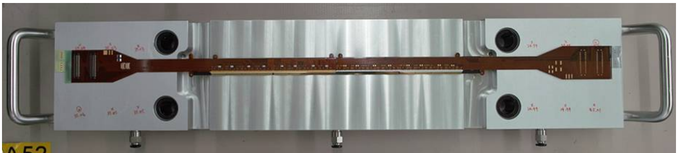
Fig. 3. Assembled full pixel ladder: It consists from one carbon fiber stave, four sensor module, and two readout buses.
