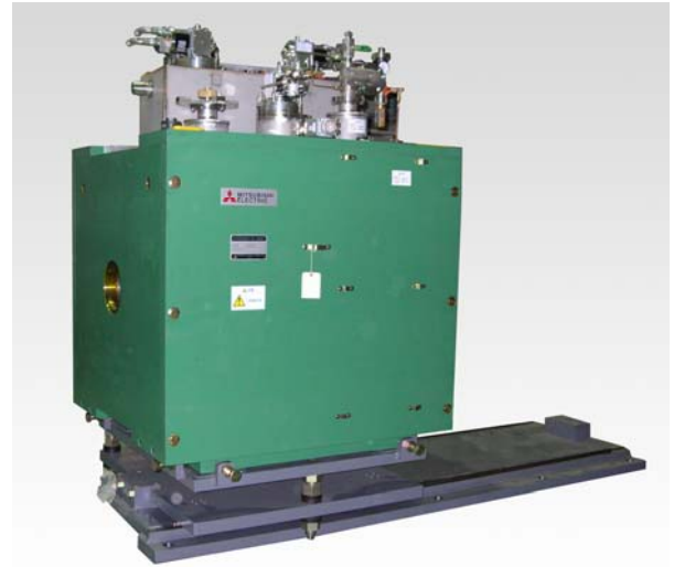
Fig. 4. Photograph of the completed superconducting magnet for the 28 GHz ECR ion source.
