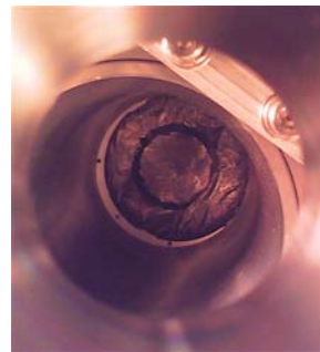
Fig. 6. Photograph of the 300 \mu\text{g}/\text{cm}^2 -thick multi-layer PCC-foil that was set in the rotating-cylinder stripper device and ruptured after 25-min beam irradiation. The ring area was discolored due to beam irradiation.
